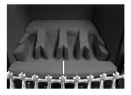
c) Fit five of the large sized coals onto the front ceramic rail, ensuring that they are evenly spaced. Use the recess's in the front ceramic rail as a guide for placement. (See fig. 3 below)
